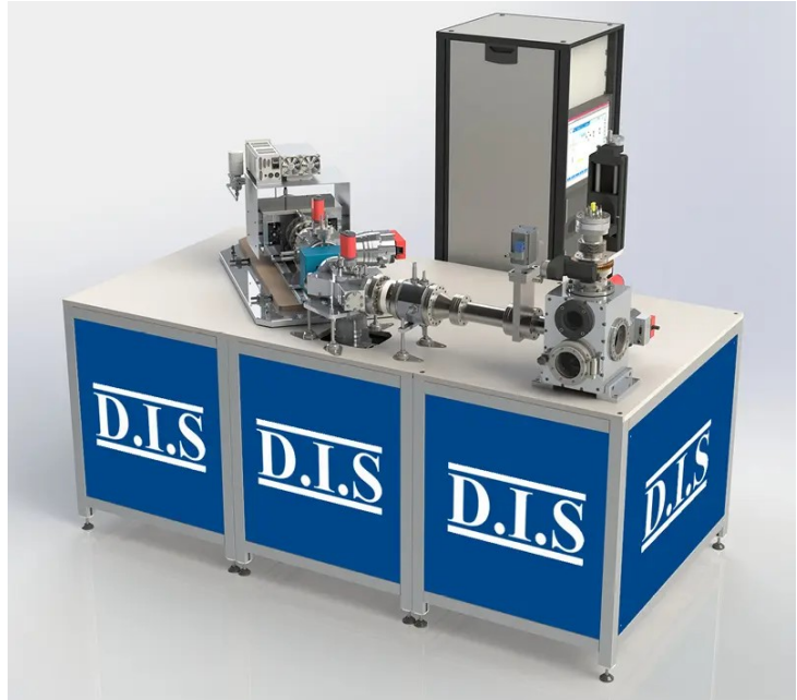
Ion Irradiation Facility, Type-M + Irradiation Chamber Setup. The electrical shielding is masked out.
